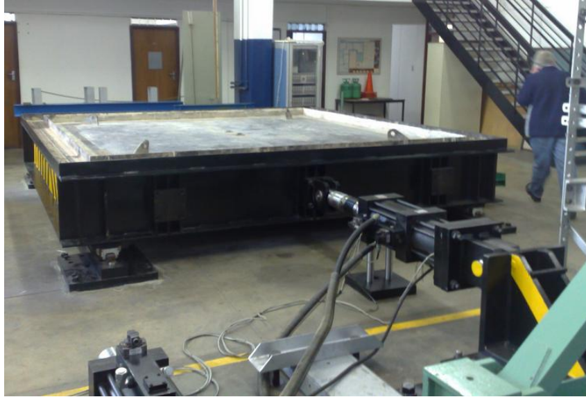
Figure 3.2 A typical shake table with hydraulic actuators
