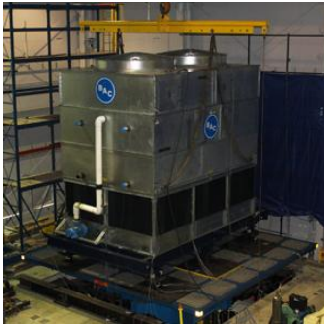
Figure 3.1 Model being tested on shake table
