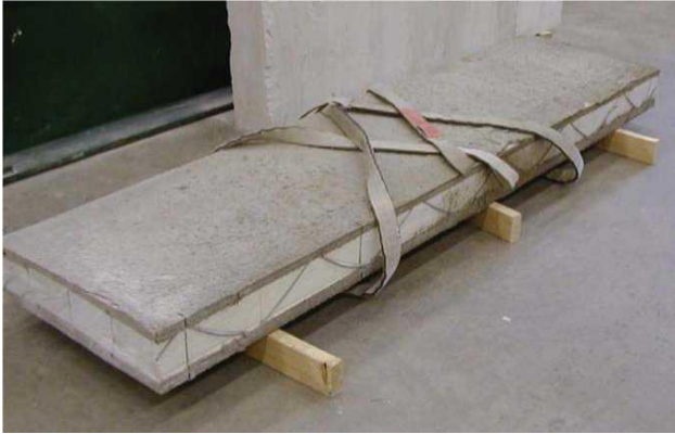
Figure 3.1: Typical SCIP System
