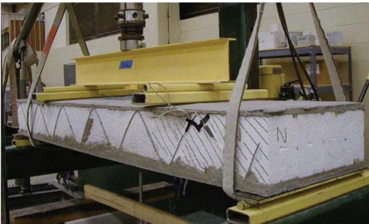
Figure 2.4: Flexural test setup [Fouad et al. (2004)]
