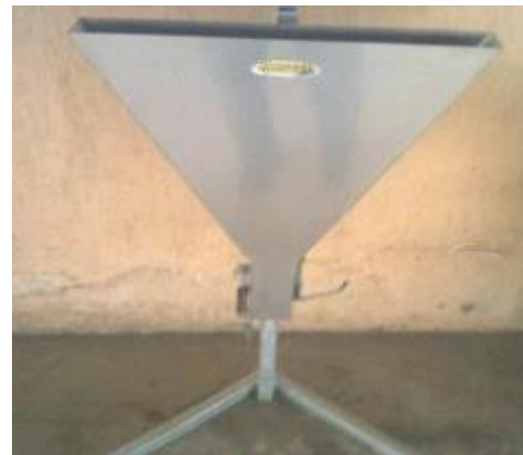
Fig. 3.7: Apparatus for V Funnel Test [64]
