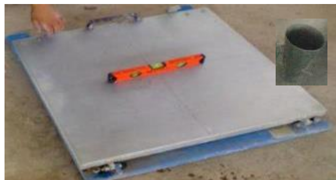
Fig. 3.6: Apparatus for Slump Flow Test [1]
