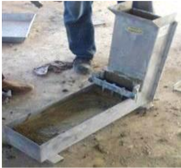
Fig. 3.8: Apparatus of L-Box
