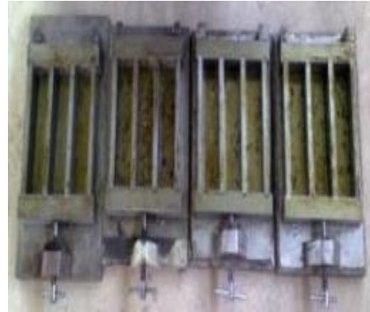
Fig 3.1 (b): Moulds of SCP Prism
