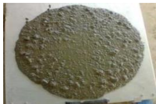
Fig. 3.9: J Ring Test
