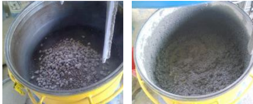
Fig. 3.5 : Preparation of SCC Mixes
