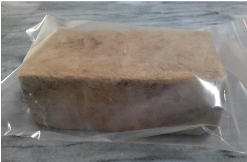
Fig 3.4: Specimen Wrapped in Polythene Bag for ASTM C 1314
