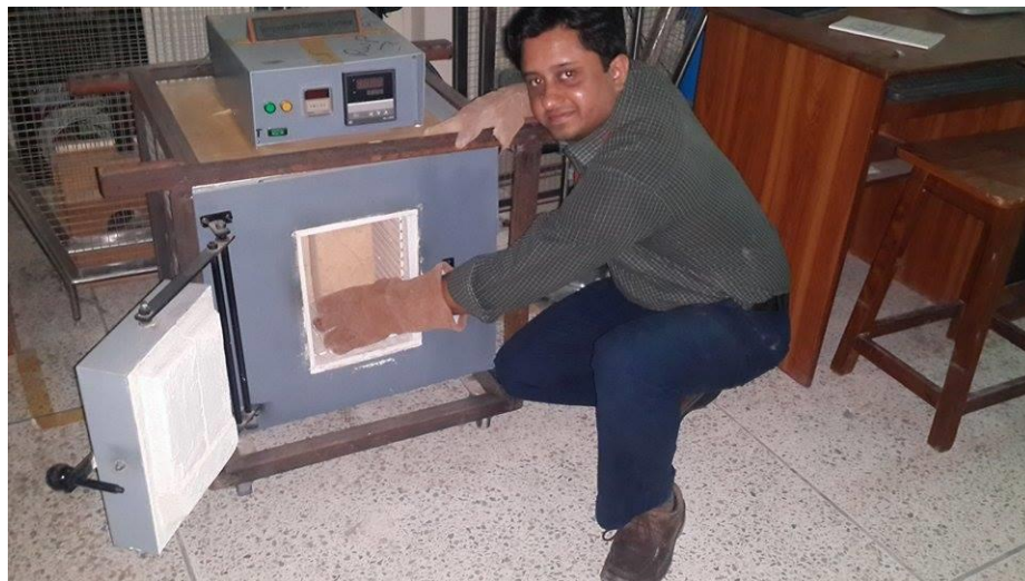
Fig 3.12: Electric Furnace with Temperature Range up to 800°C
