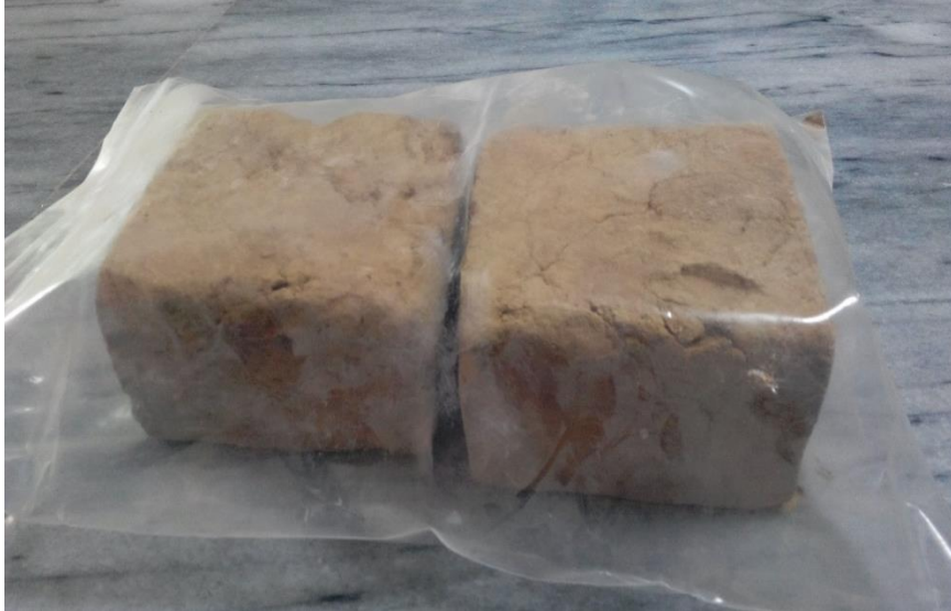
Fig 3.3: Specimen Wrapped in Polythene Bag for ASTM C 1314
