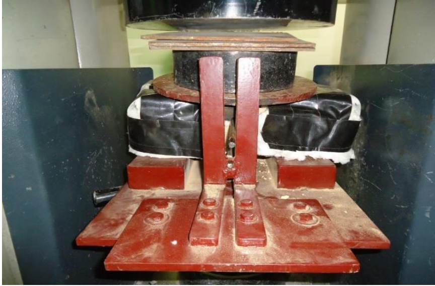
Fig 3.5: ASTM C 1006 Splitting Tensile Strength Apparatus
