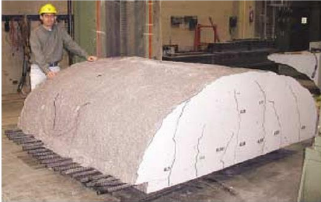
Figure 2.8: Failure surface of beam AT-1 (Lubell et al. 2004).
