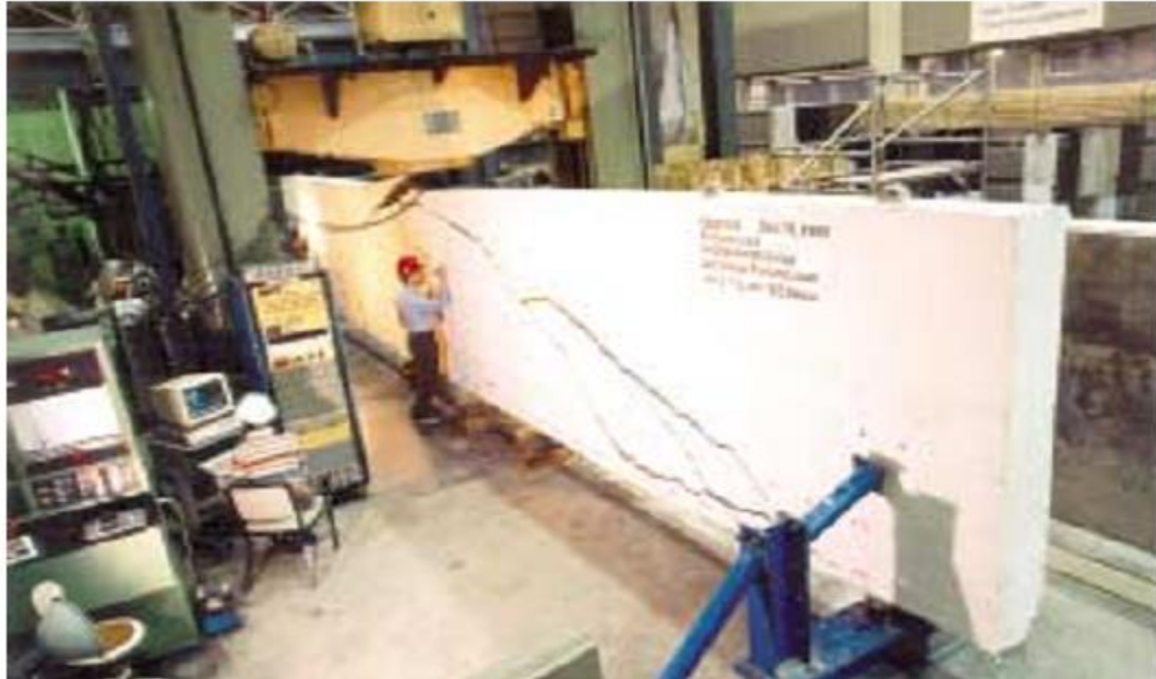
Figure 2.2: Failure of large beam at 47% of ACI shear failure loads (Lubell et al. 2004).
