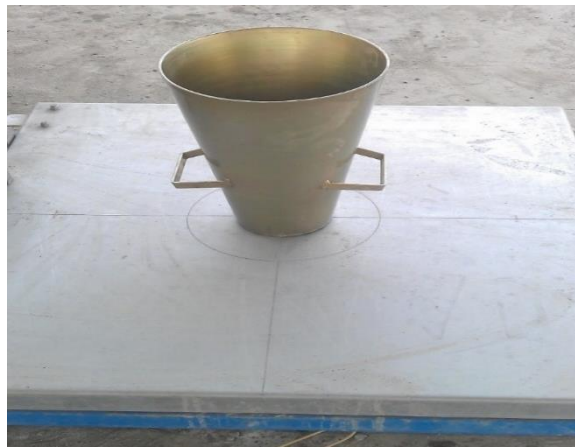
Figure 3-6: Slump Flow Test for SCC using Abrams Cone of 100x200x300 cm 3 (top end down)
