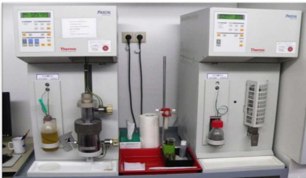
Figure 3-18: Mercury Intrusion Porosimeter at TU Freiberg Germany Pascal 140 (Right) and Pascal 440 (Left)
