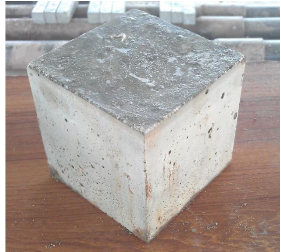
Figure 3-14: Demoulded Cube (BS EN 12390-1)
