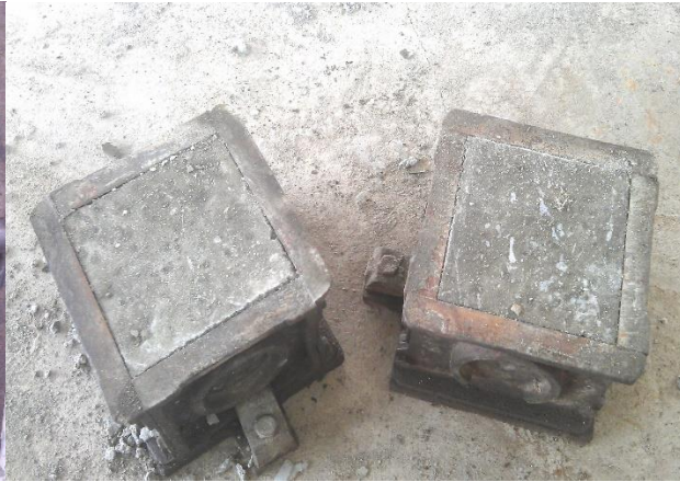
Figure 3-12: 4x4x4 inch 3 Cubes for Self-compacting Concrete (BS EN 12390-1)
