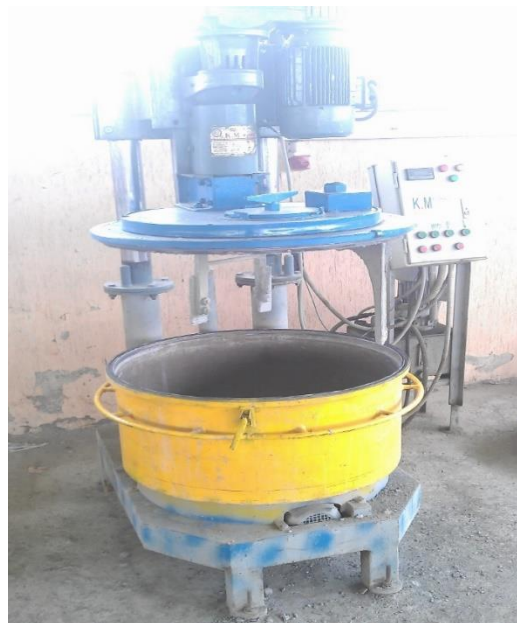
Figure 3-5: Indigenous local High Performance Concrete Pan Mixer developed at NICE
