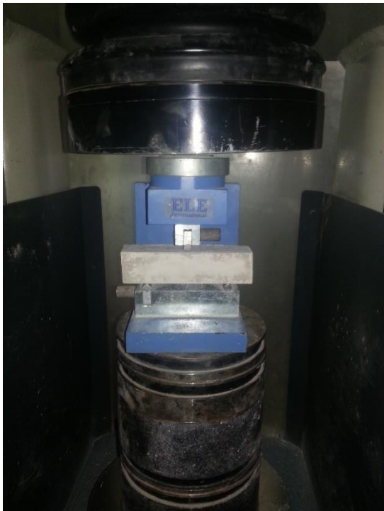
Figure 3-15: Flexure & Compression Testing Assembly for Prisms using Controls 500 kN Compression Testing Machine
