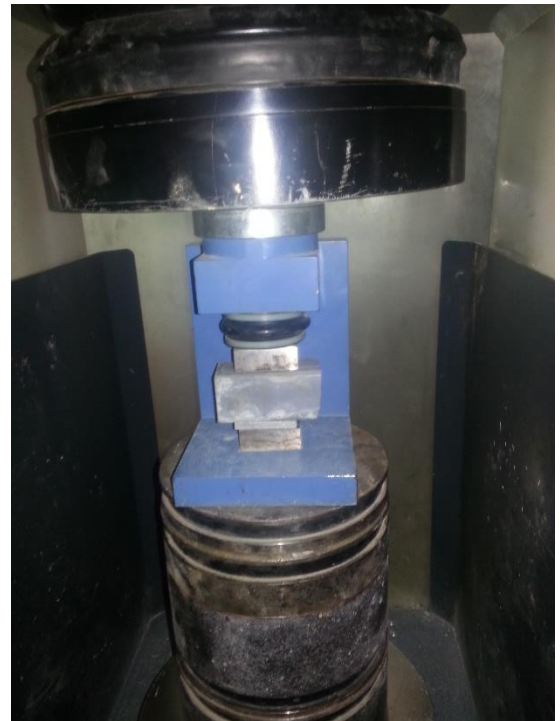
Figure 3-15: Flexure & Compression Testing Assembly for Prisms using Controls 500 kN Compression Testing Machine
