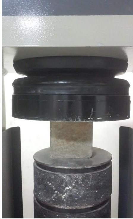
Figure 3-16: Compression Testing Assembly for Cubes using Controls 500 kN Compression Testing Machine at NICE Structures Lab
