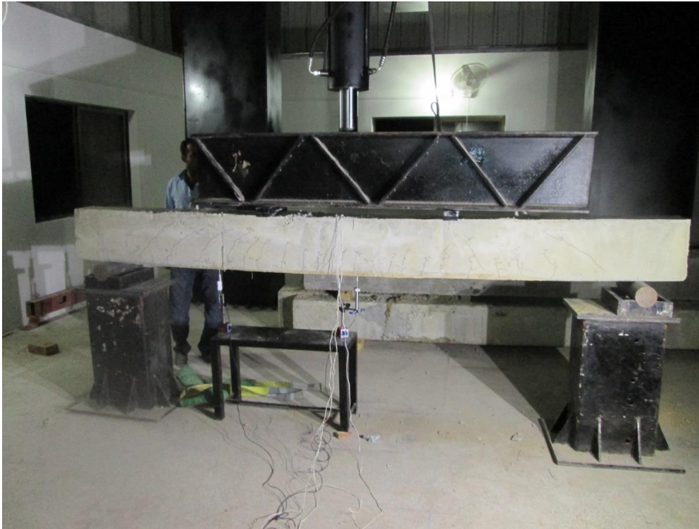
Figure B-8 : Loading Arrangement
