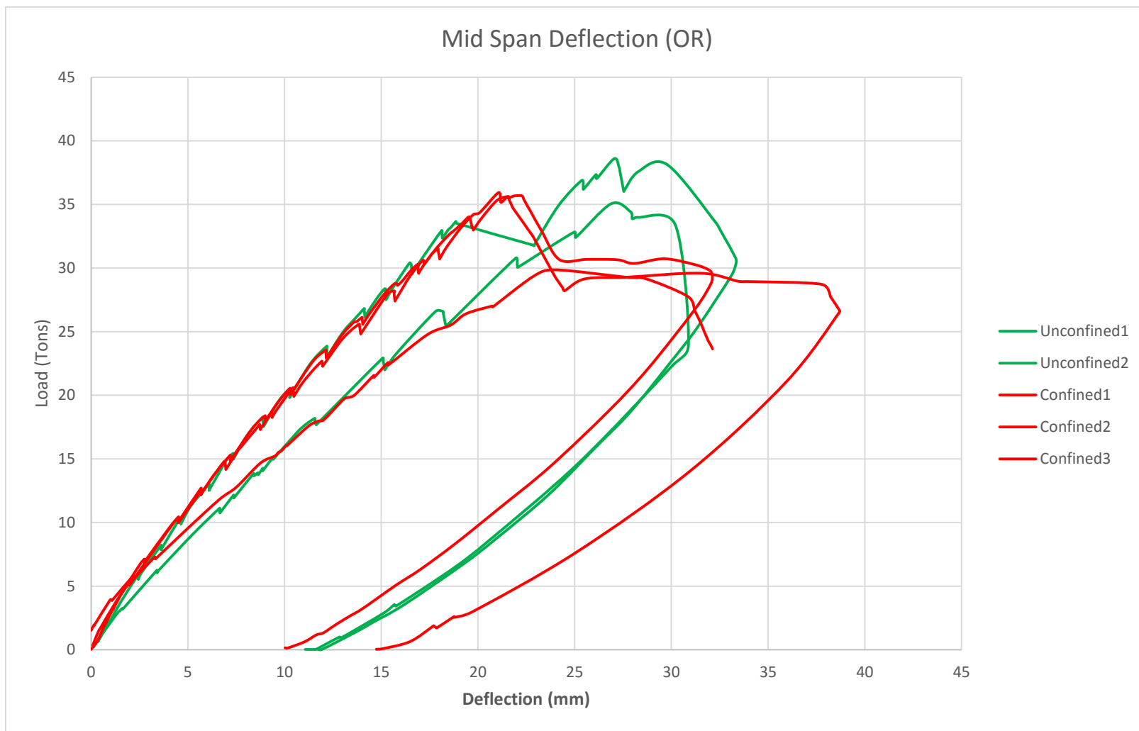
Figure 0-2: Load Deflection Comparison of Over reinforced confined and unconfined Beams
