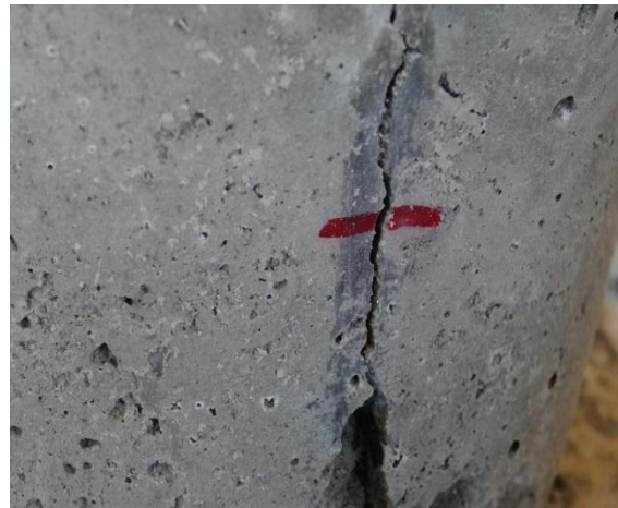
Fig. 3.7 Marking of cracks on pre-cracked specimens to ensure that multiple reading are taken from the same point
