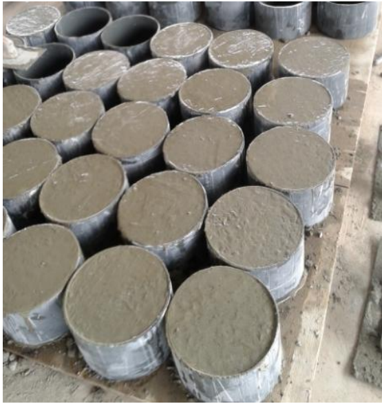
Casting of samples for pre-cracking
