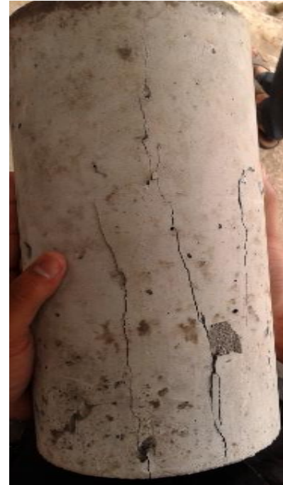
Cylinder after compressive strength test
