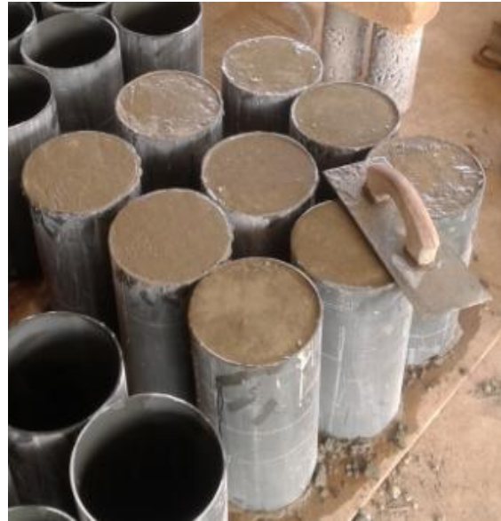
Casting of samples for compressive strength measurement
