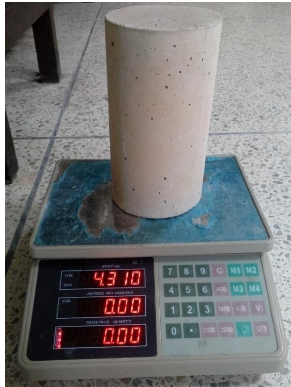
Figure 3.10 – Cylinder being weighed after exposure to elevated temperature.
