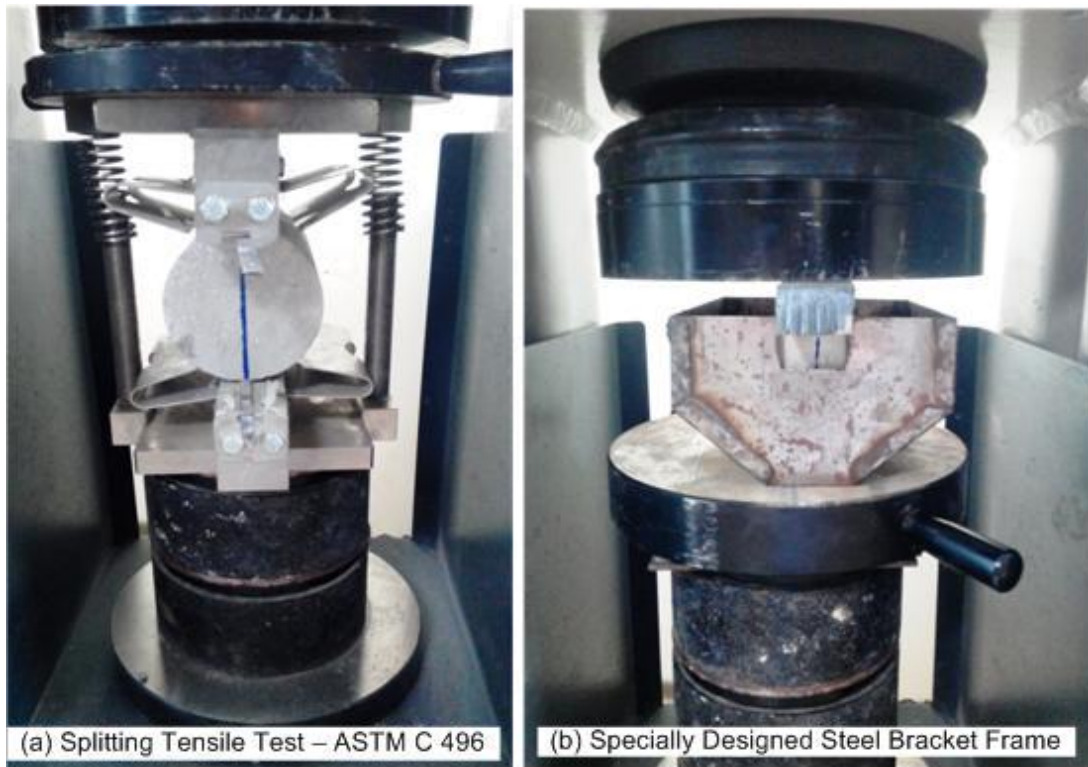
Figure 3.9 – Samples ready for split tensile strength test at room temperature.
