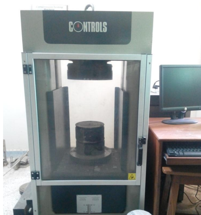
Figure 3.5 – Controls strength test machine used for mechanical properties.
