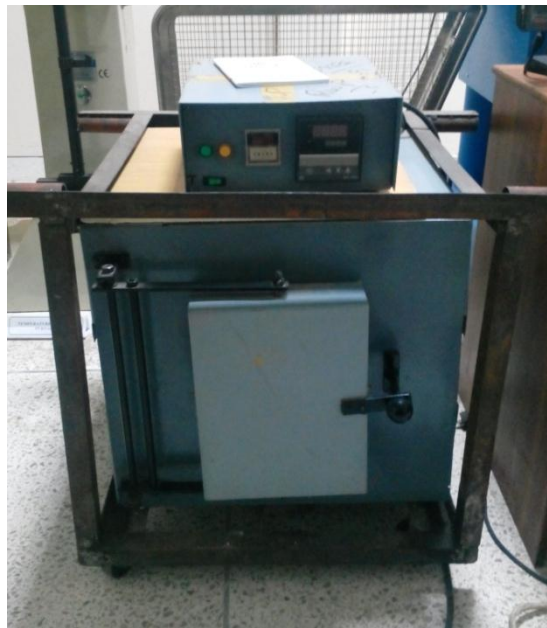
Figure 3.4 – Electric Furnace used to heat the concrete cylinders.
