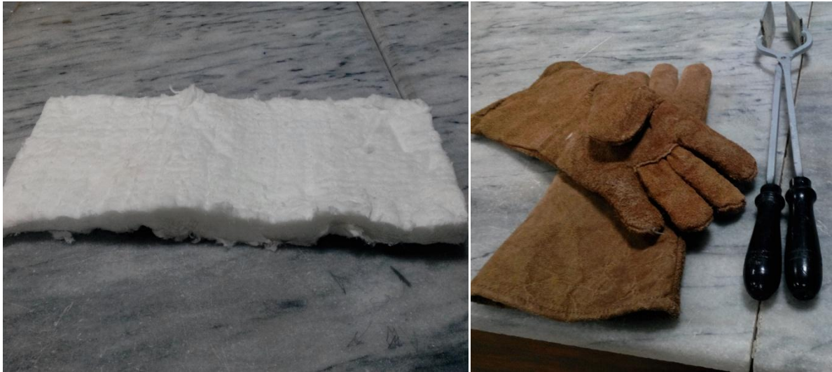
Figure 3.6 – Thermal jacket and safety equipment for handling the heated cylinders.
