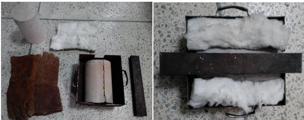
Figure 3.8 – Insulated steel bracket frame for handling and preserve the heat in cylinders during splitting tensile strength tests.
