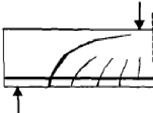
Figure 2-5 : Diagonal tension failure
