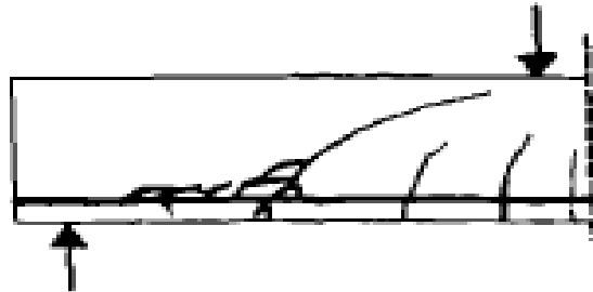
Figure 2-6 : Shear tension failure
