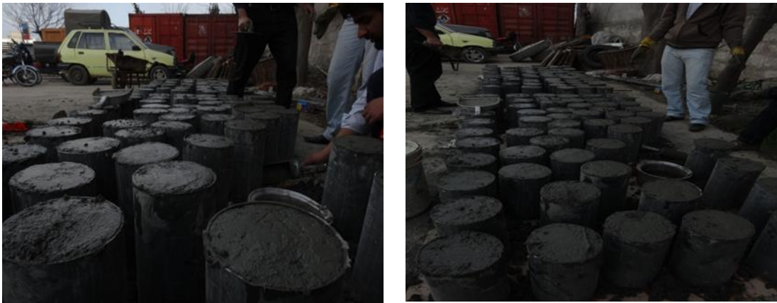
Fig 3.3 Casting of specimens
