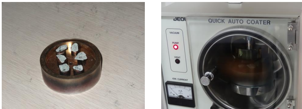
Fig 3.5 Sample preparation for SEM analysis
