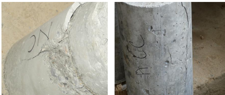
Fig 3.4 Cracking pattern of NC and ACC specimens
