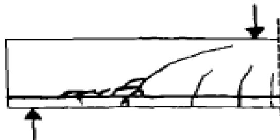
Figure 2- 6 Shear tension failure
