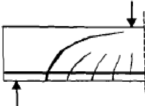
Figure 2- 5 Diagonal tension failure
