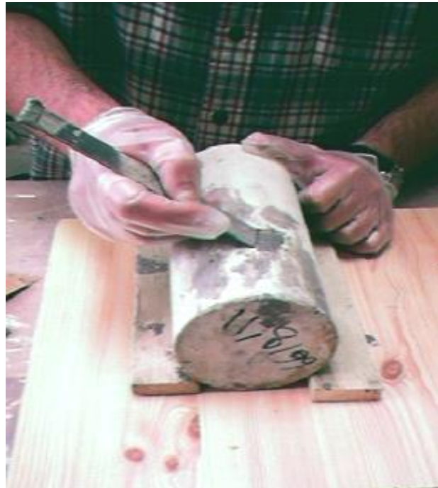
Figure 3-3 Filling the gaps
