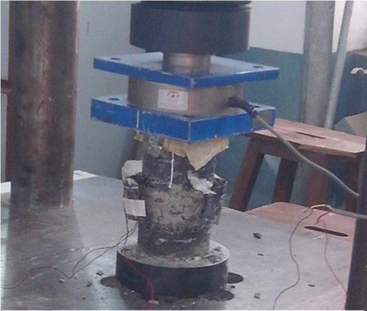
Figure 4-3 Failed confined specimens by wrapping with CFRP
