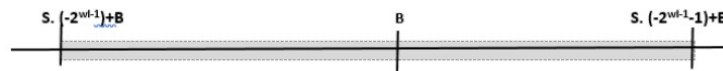
Figure 2.4: Fixed-point numbers for signed and unsigned data type, the distinct bit patterns is 2^{wl} .
