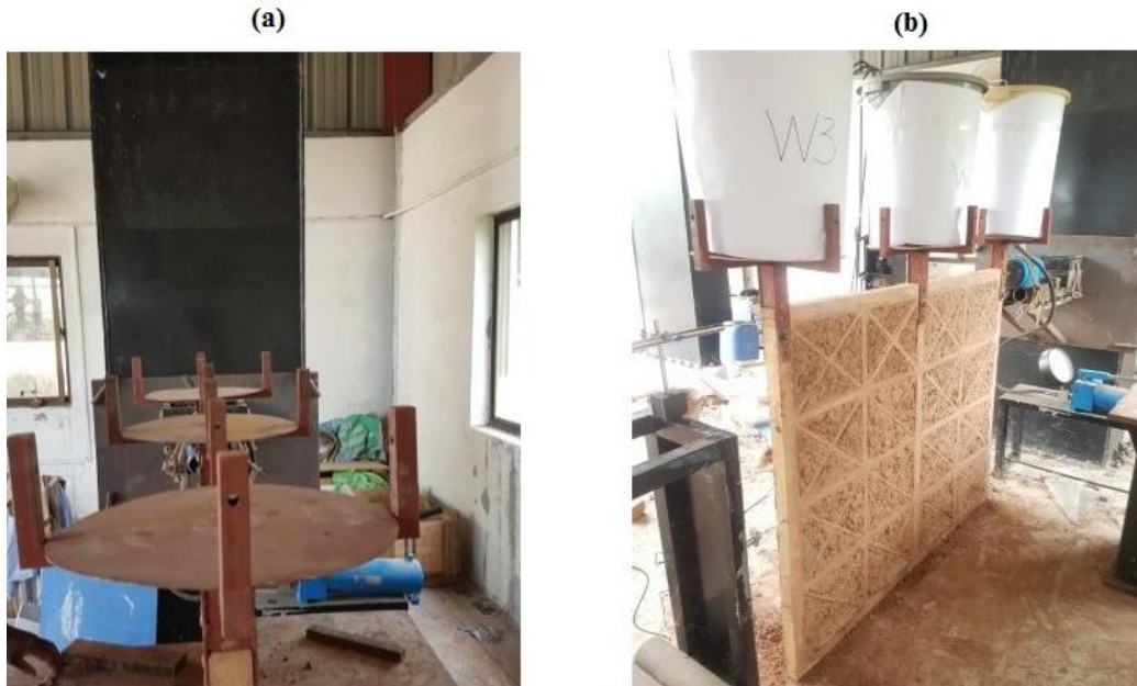
Fig 3.6: (a) Iron Moulds (b) Application of Load
