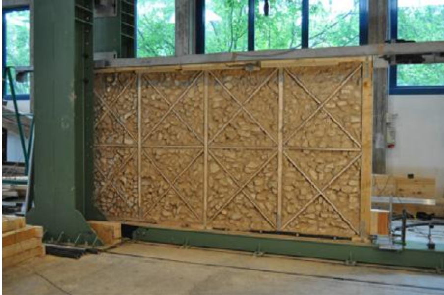
Fig 2.17: Traditional wall tested by Vieux [26]
