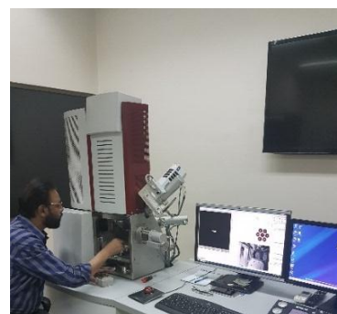
Figure 3.13 Sample Placement in SEM chamber
