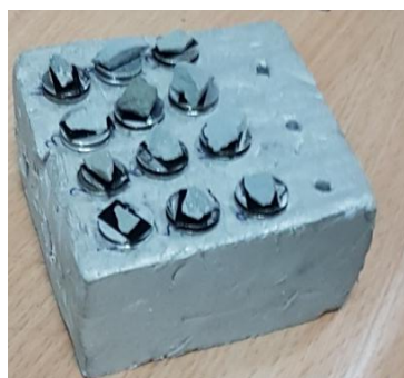
Figure 3.11 Samples wrapped in conductive tape
