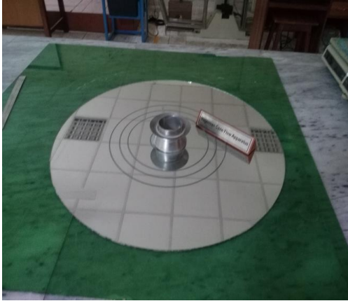
Figure 3.4 Hagerman's mini-cone slump apparatus
