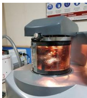
Figure 3.12 Sputter coater for carbon coating of the samples
