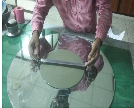
Figure 3.5 Orthogonal Diameter measurement
