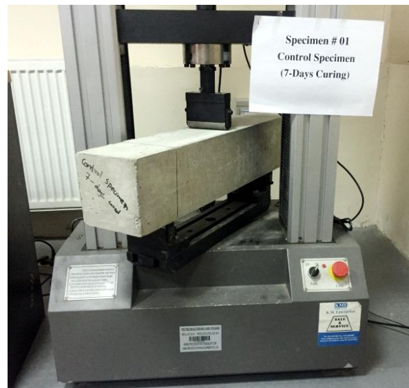
Figure 3.13: Strain controlled three-point bend test arrangement on concrete specimen
