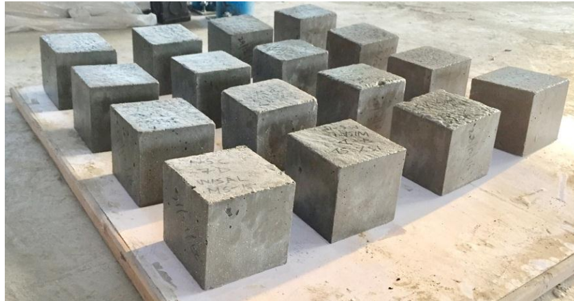
Figure 3.10: Concrete cubes ready for compression test
