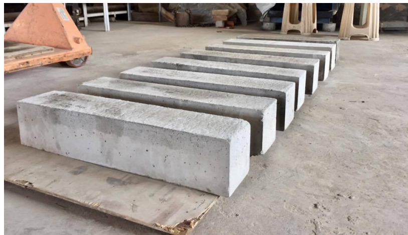
Figure 3.11: Concrete prisms after 7-days of curing
