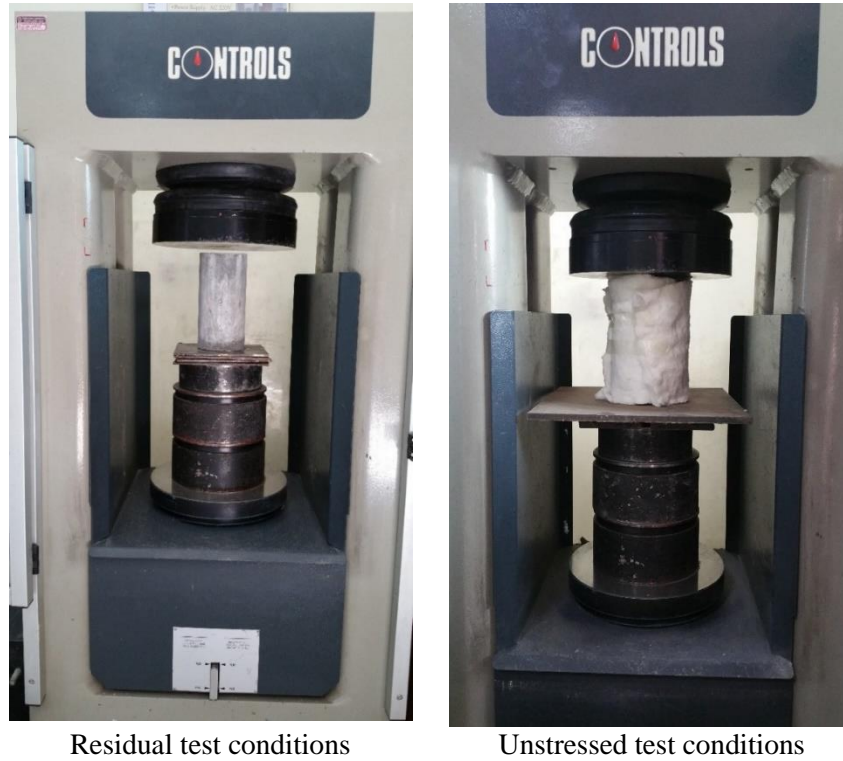
Fig. 3.10 Compressive strength test under action
