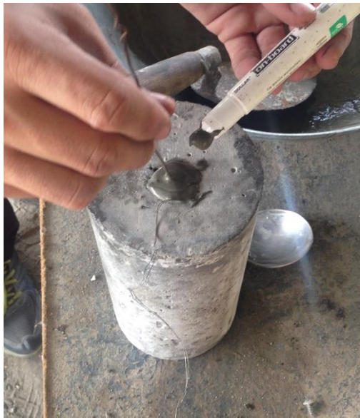
(a) Thermocouple being embedded in concrete cylinder
