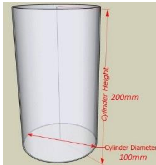
Fig. 3.7 Cylinder size and dimensions
