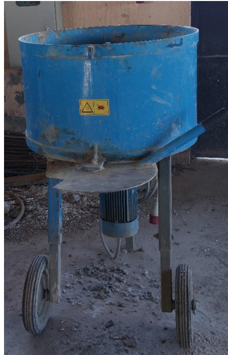
Fig. 3.4 Horizontal concrete mixture
