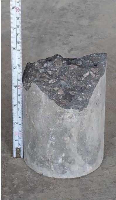
Fig. 4.1 Spalling of NAEH-1 mixture specimen
