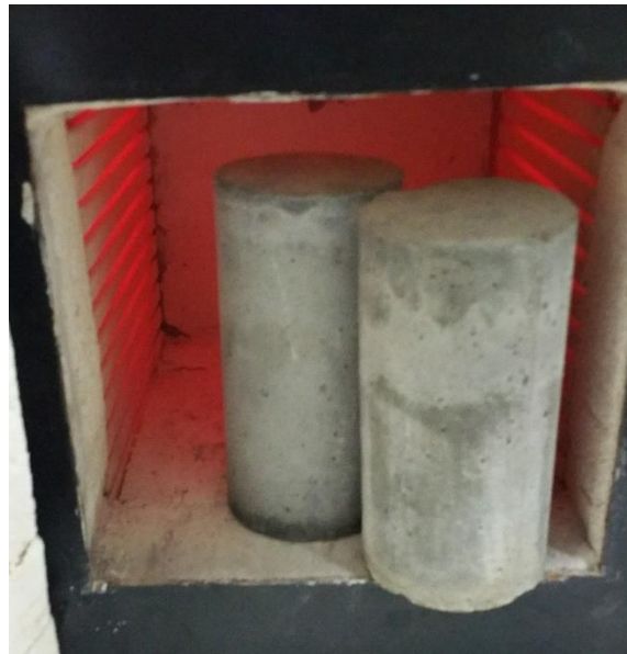
Fig. 4.2 Spalling (explosive) of NAEH-2 mixture specimen
