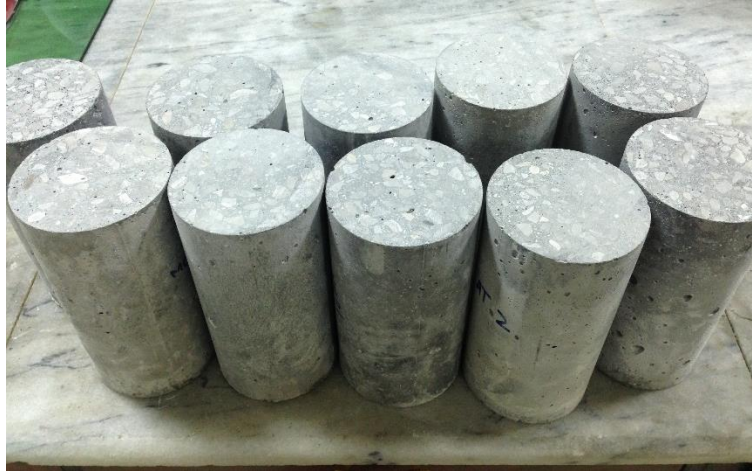
Fig. 3.6 Concrete specimens with ground ends
