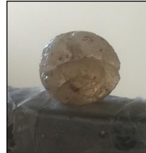
Figs 4.6 (c) Day 5 – Lumps retain their shape and become stiffer with time.
