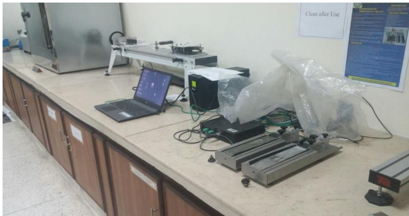
Fig. 3.3: German Schwindrine apparatus
