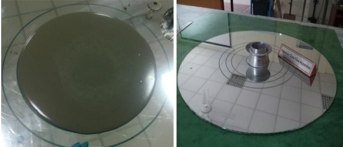
Figure 3.6: Hagerman's mini slump cone
