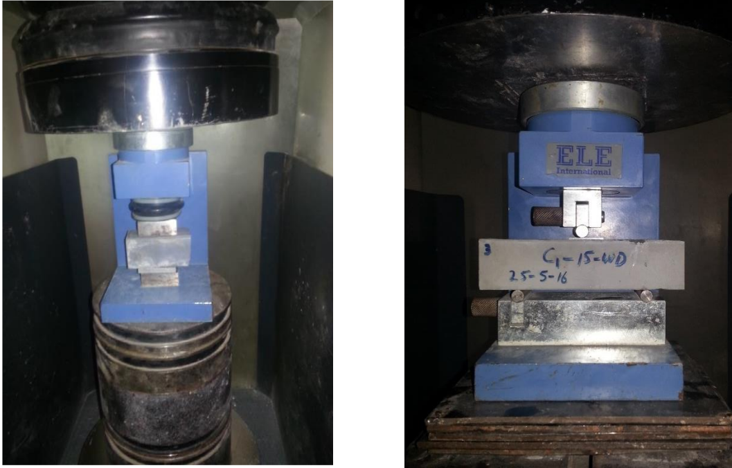
Figure 3.10: Assembly for compression and flexure testing
