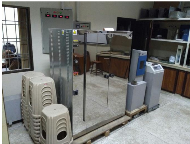
Figure 4: Oven used for drying fine aggregate
