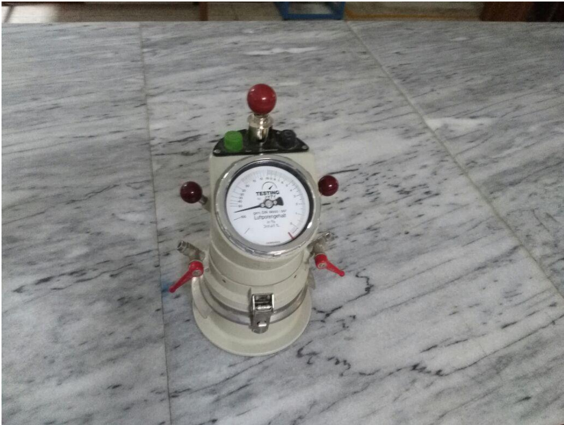
Figure 18: Luftporengehalt apparatus used to calculate air content of SCM formulations containing RHAP and RHAG
