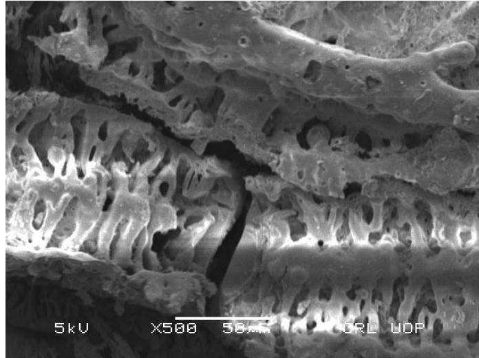
Figure 2: SEM image of RHA Particle
