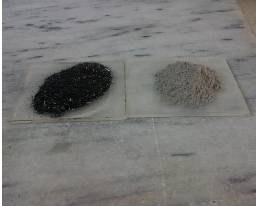
Figure 6: RHAG-81 (Left) and RHAP-21 (Right) powders
