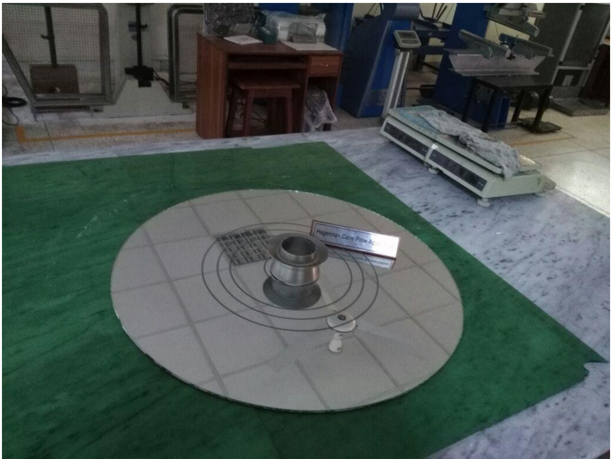
Figure 22: Haggerman's cone for measure the spread of SCM formulations
