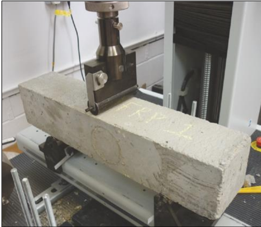
Figure 3-10: Flexure test setup (three-point bend test)
