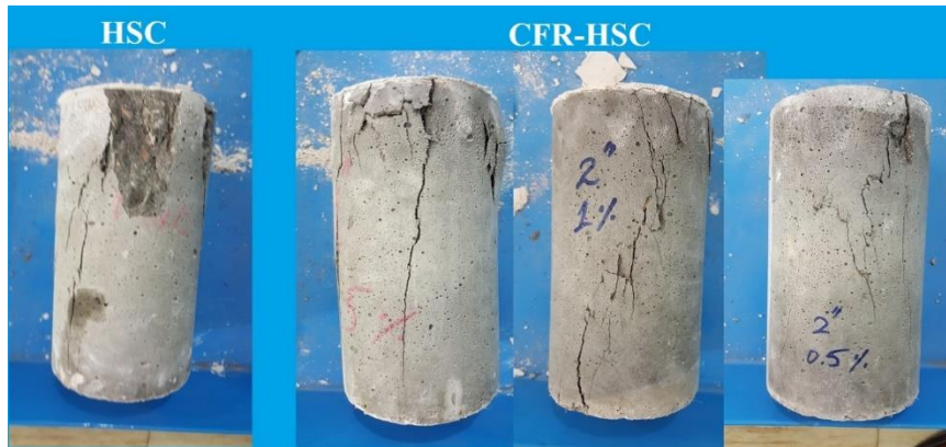
Figure 4.5: HSC and CFR-HSC specimens after compressive strength tests
