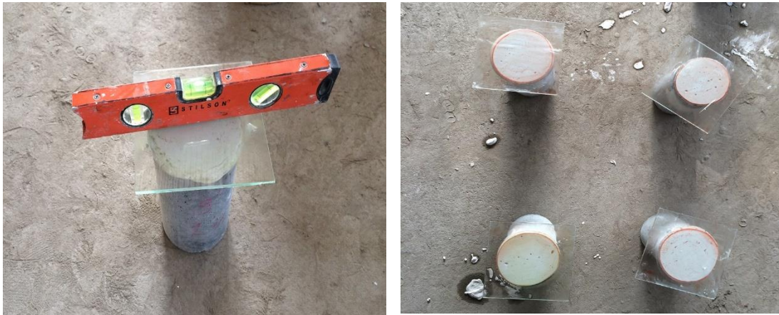
Figure 3.5: Capping of cylinders
