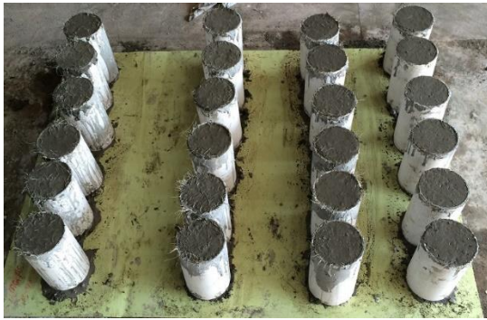
(a) Casted cylinders in molds
