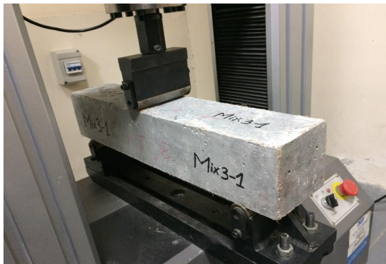
Figure 3.8: Arrangement of 3-point load test for beams
