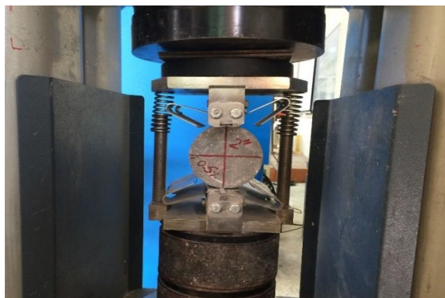
Figure 3.7: Splitting tensile strength test setup
