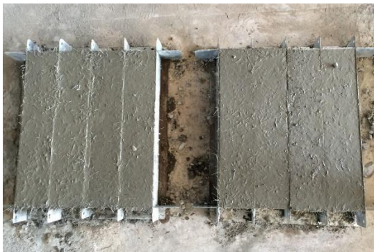
(c) Casted beams in molds
