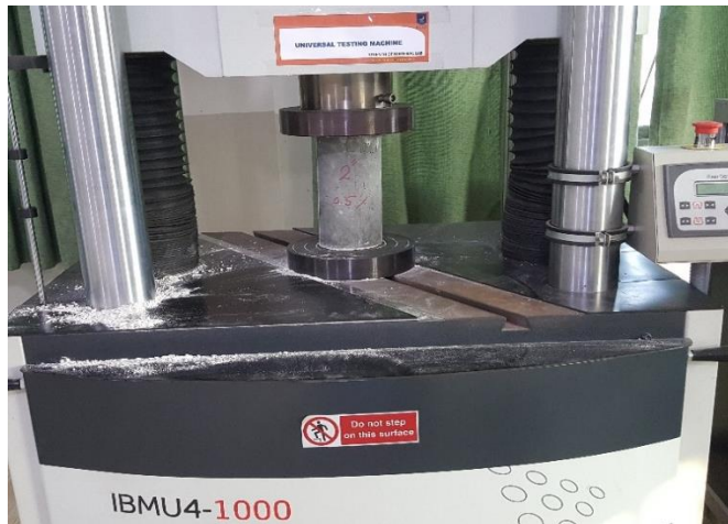
Figure 3.6: Compression testing of cylinder in UTM
