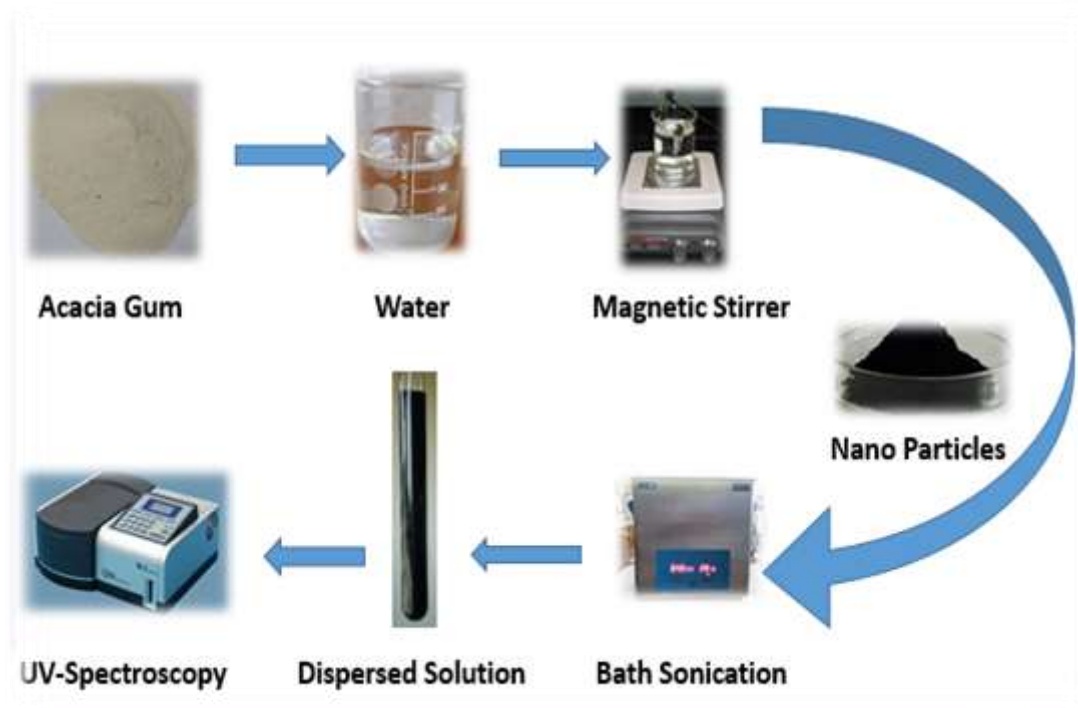
Figure 3-1 Schematic Diagram for Dispersion of Nano Materials in Aqueous Solution
