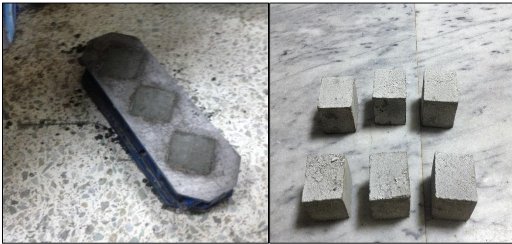
Figure 3.7 Casting of samples
