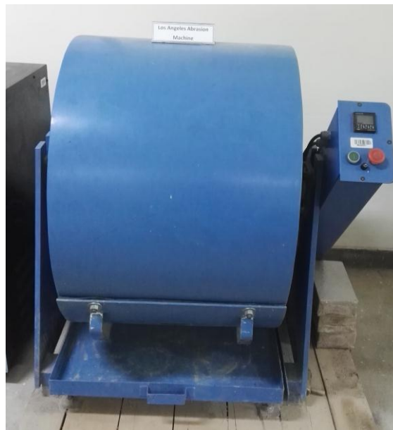
Figure 3.2: Los Angeles Abrasion Machine
