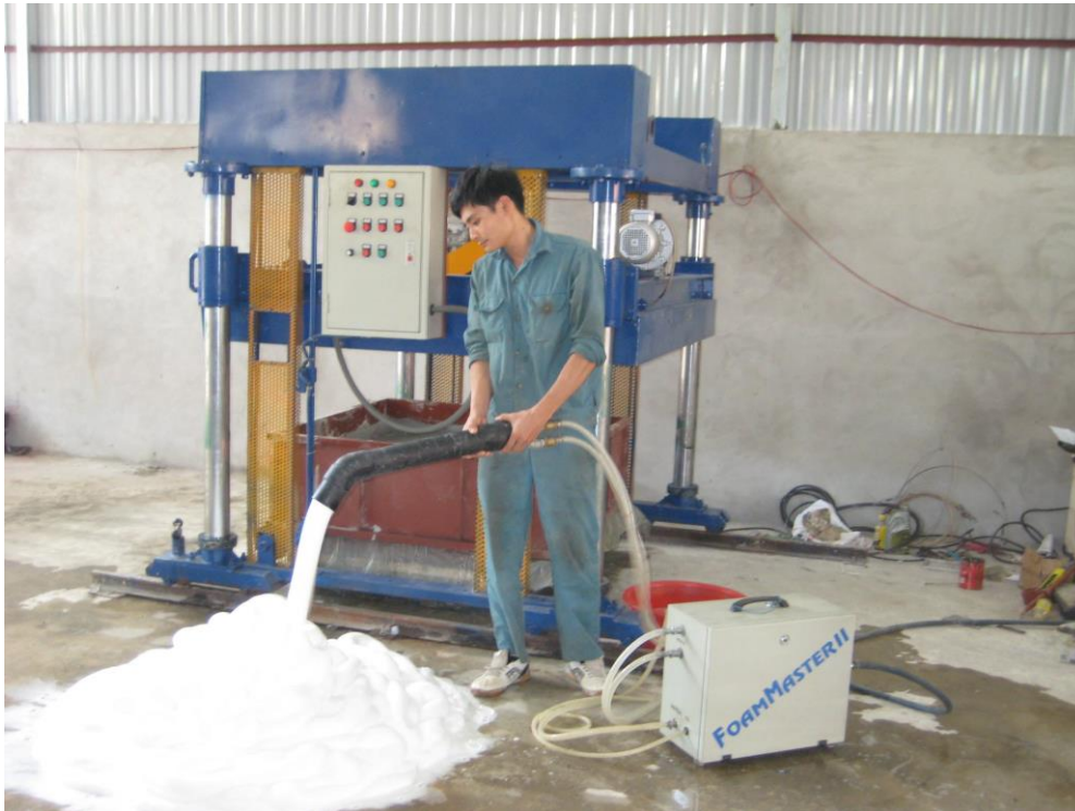
Fig 3.2: Worker making foam using foam generator machine in the field.
