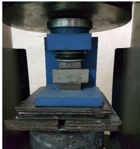
Fig. 3.10(a) Assembly for Compression in UTM
