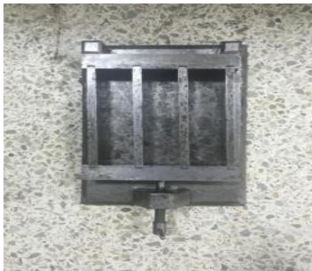
Fig. 3.9 (a) 160x40x40 mm moulds (Empty)
