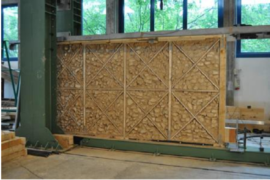
Fig 2.126: Traditional wall tested by Vieux [38]
