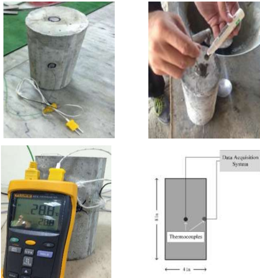
Figure 3.10 Instrumentation procedure for determining heating characteristics of each mix
