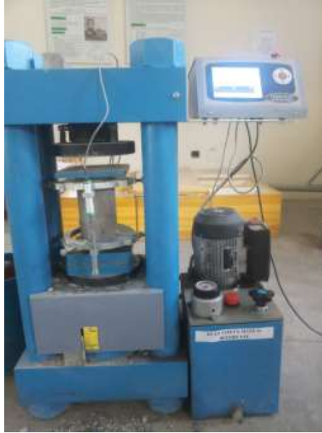
Figure 3.12 Compressive Strength testing of specimen
