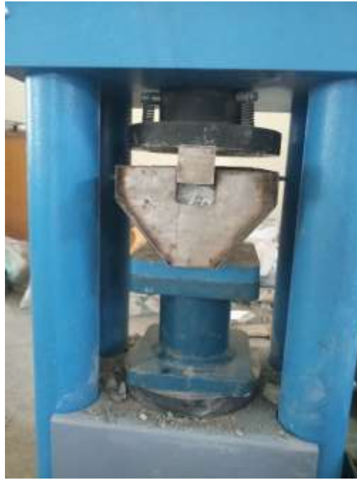
Figure 3.13 Splitting tensile strength test
