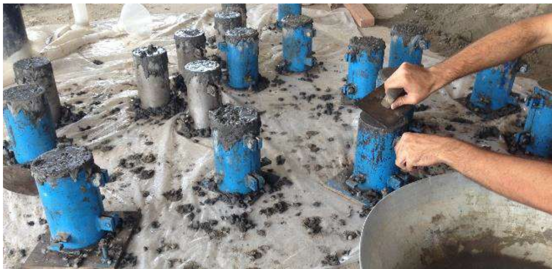
Figure 3.7 Concrete cylindrical specimens casting
