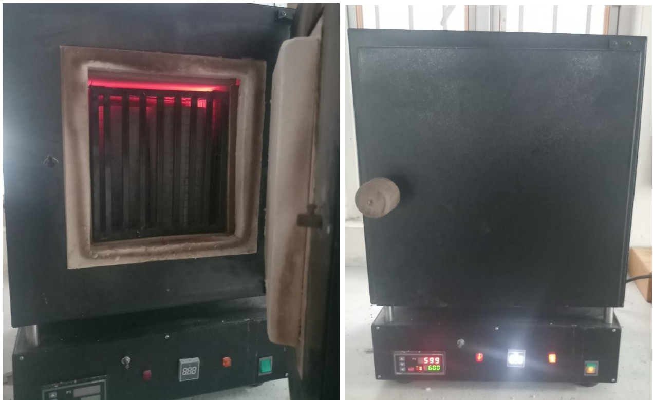
Figure 12 : Electric Furnace for heating the samples to targeted temperatures
