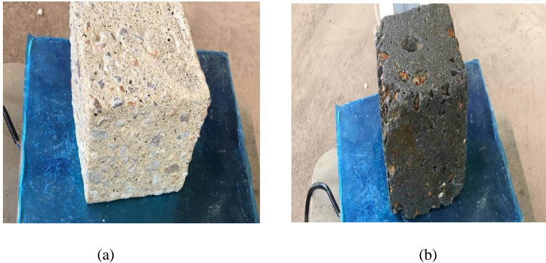
Figure 3-4: Specimen (a) after sulfate attack (b) after HCL attack
