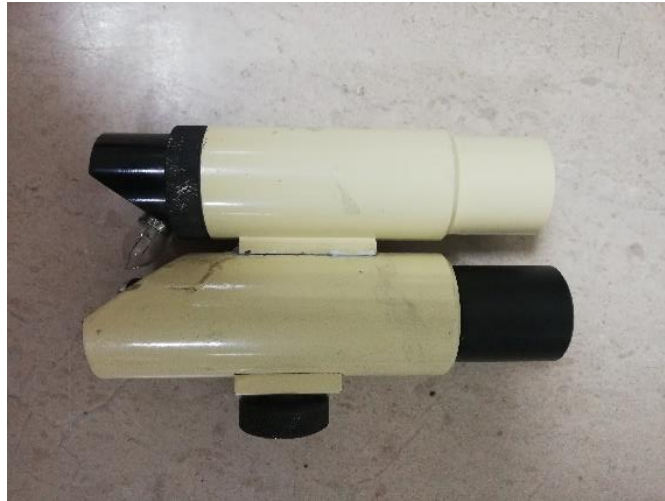
Figure 3.21: Crack width measuring microscope
