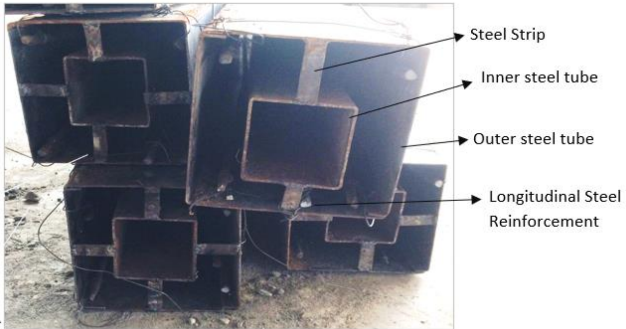
Figure 11: Fabrication of specimen
