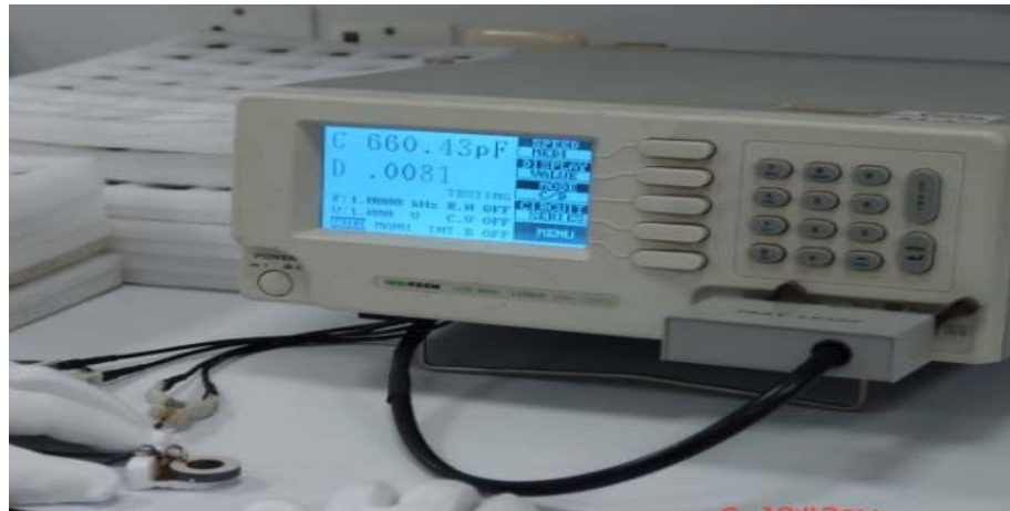
Figure 4.1 A LCR meter used to measure dielectric properties.
