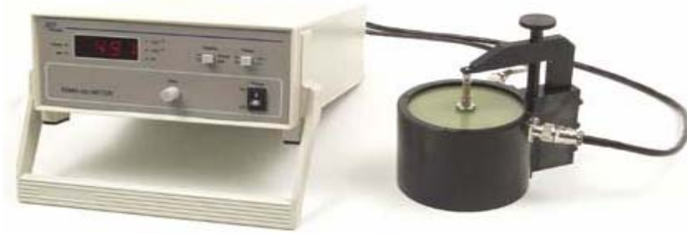
Figure 4.4 A typical d_{33} meter employed to measure charge coefficient d_{33} .
