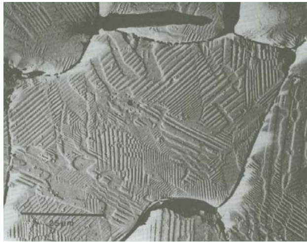
Figure 3.5 Polished and etched surface of unpoled ceramic.
