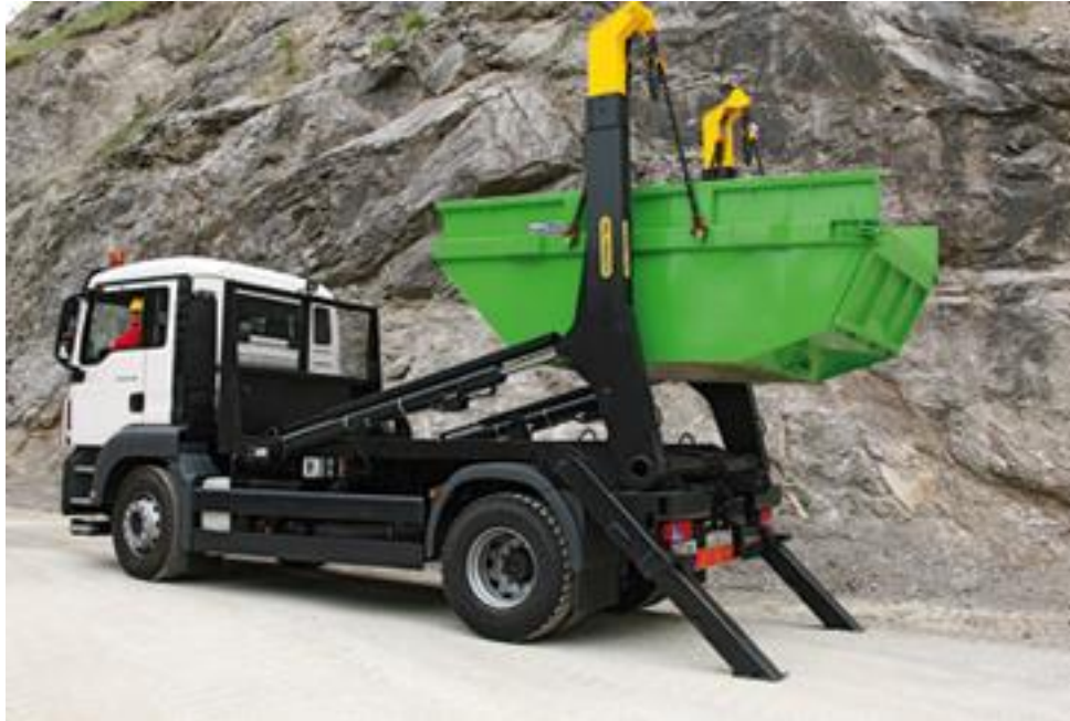
Figure 16: Truck used for automatically loading Smart dumpsters
