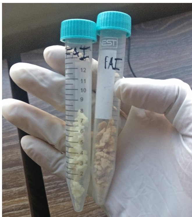
Figure 15: R to L: FAI crystals before washing and FAI crystals after washing with diethyl ether
