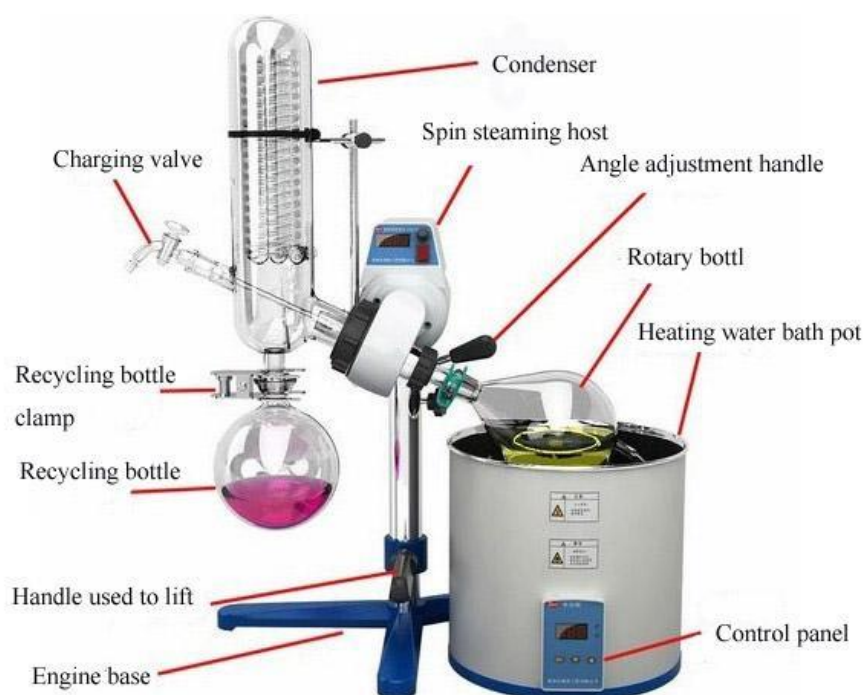
Figure 7: Labelled diagram of a rotary evaporator setup [1]
