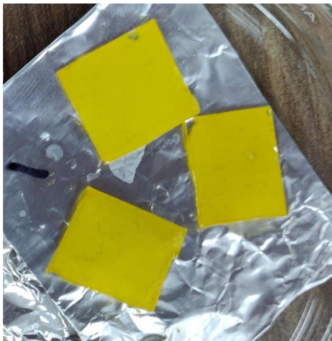
Figure 16 \text{PbI}_2 films after deposition and annealing
