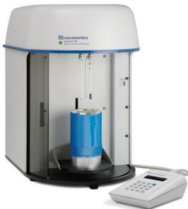
Figure 5.3 Gemini® VII 2390 Micro porosity analyzer
