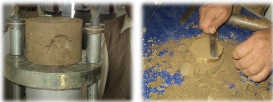
Figure 3.3 The undisturbed sample were later ejected carefully from the Shelby tubes using hydraulic jacks and carefully trimmed sample were cut for different tests.
