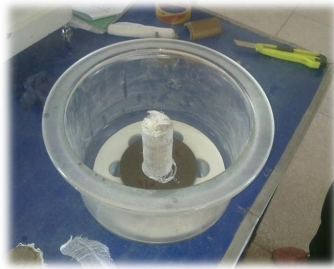
Figure 3.6 UCC samples before and after 24hrs for soaking.
