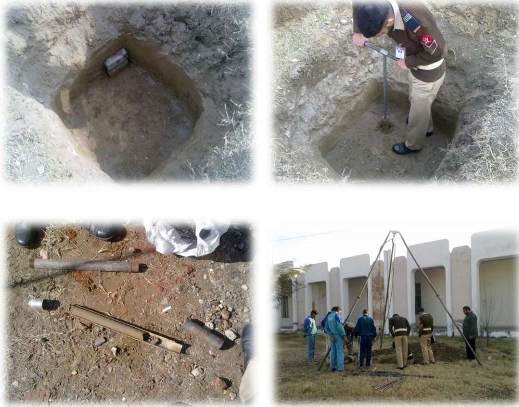
Figure 3.1 A view of test pit #1 and collection of disturbed samples using split spoon samples.
