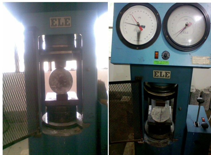
Figure 3.11: Splitting Tensile Test
