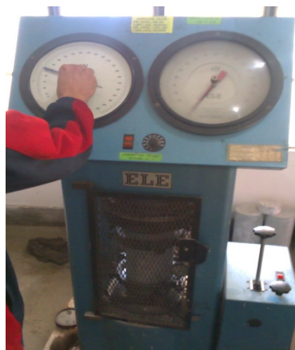
Figure 3.15. : Setting Concrete Cylinder for Testing Modulus of Elasticity
