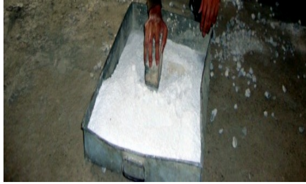
Fig 3.2: Removing Lumps from Slurry
