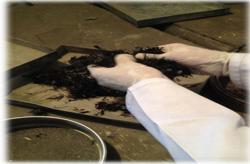
Figure 4.1 Dispersion of carbon micro fiber
