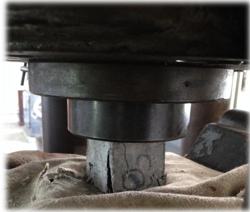
Figure 6.1 Compressive strength of the mortar cubes of 2”
