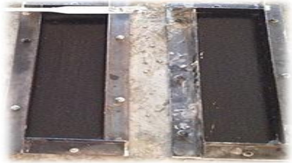
Figure 5.2 special mold 16"x4"x1.5"
