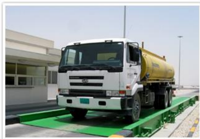
Figure 3-5: A truck using STATIC weight sensor
