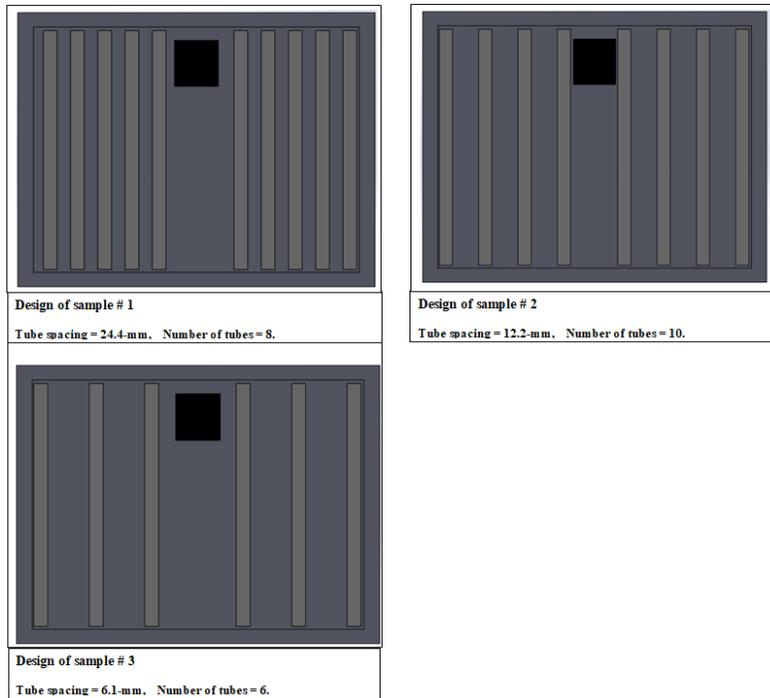
**Figure 4-1: Design of different samples in cad model**
