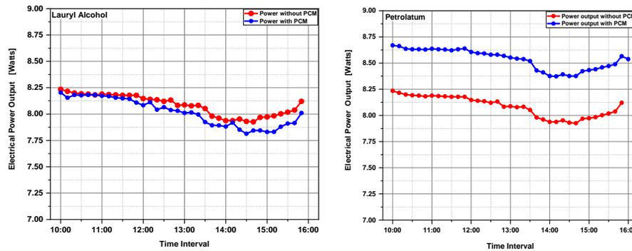
Figure 5-9: Electrical power output of PV and PV-PCM system
