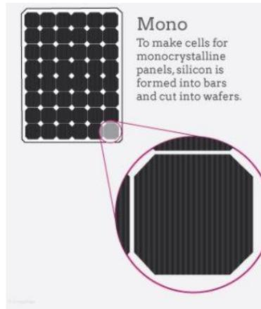
**Figure 2-1 Monocrystalline PV module [12]**
