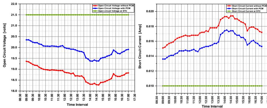
Figure 5-7: Electrical improvement in terms of open-circuit voltage and short circuit current
