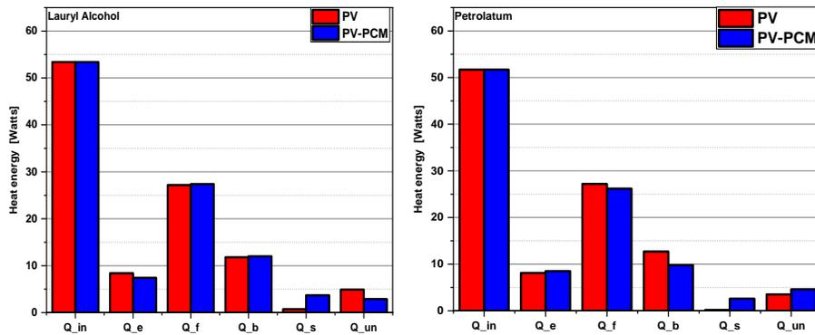
Figure 5-10: Energy balance of PV module with and without PCM
