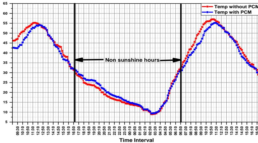
Figure 5-4: Temperature curves of the PV module with and without PCM (Lauryl Alcohol)
