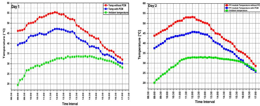
Figure 5-5: Temperature curves of the PV module with and without PCM (Petrolatum)
