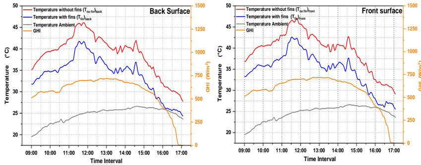
Figure 5-2: Effect of solar radiations on the surface temperature of the PV module
