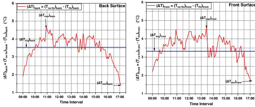
**Figure 5-1: The temperature difference between PV module with and without fins**
