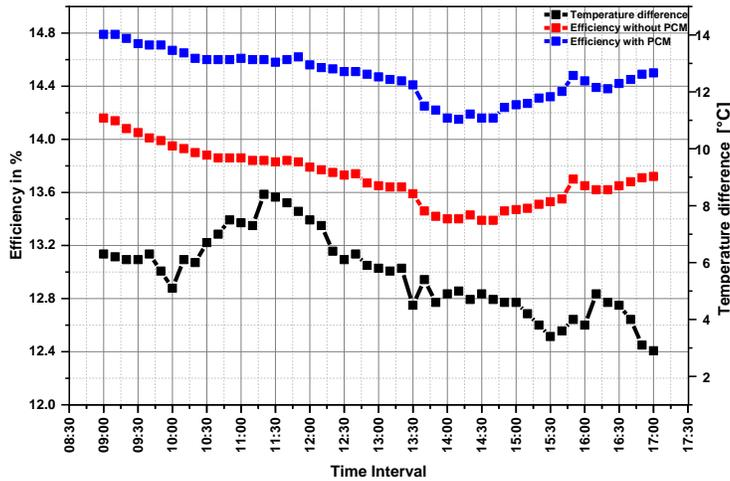
Figure 5-8: Electrical output efficiency comparison between PV module with and without PCM
