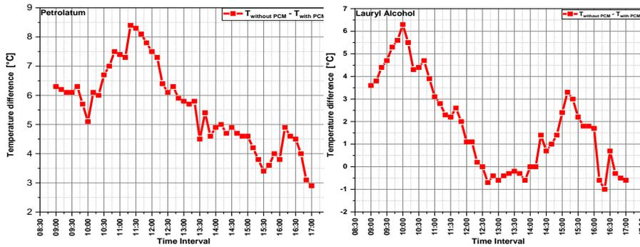
Figure .5-6: Cooling of PV module comparison between Lauryl alcohol and Petrolatum
