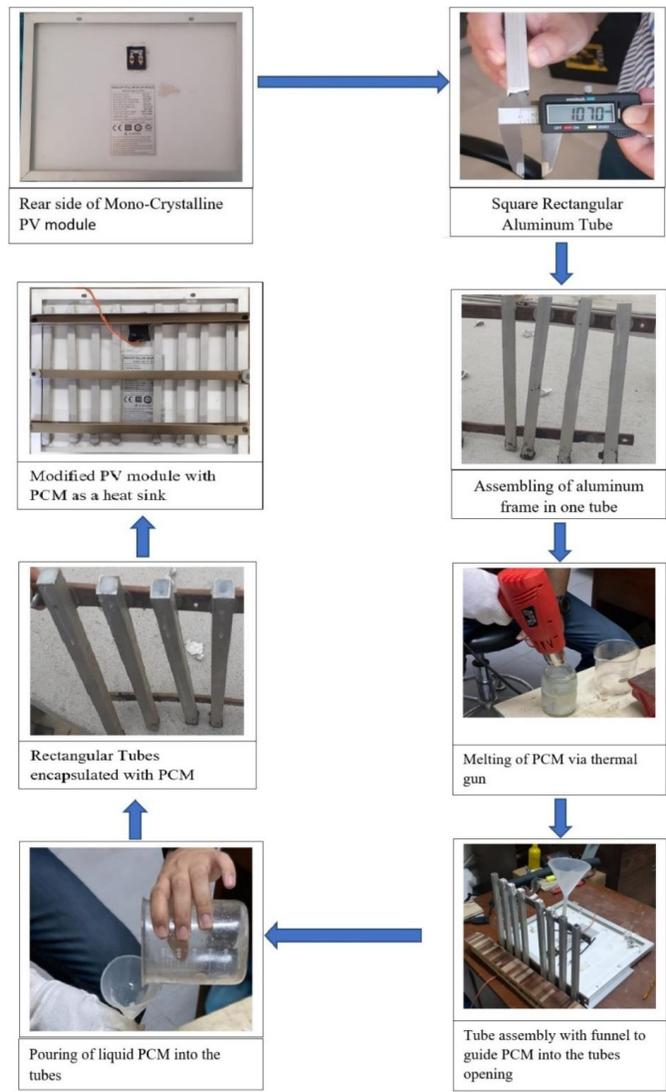
Figure 4-2: Step by step process of prototype fabrication
