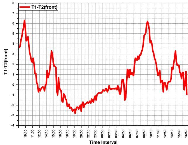
**Figure 5-3: The temperature difference between PV module with and without PCM**
