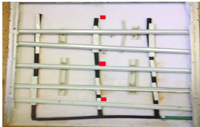
Figure 2-6: Backside water cooling system[24]
