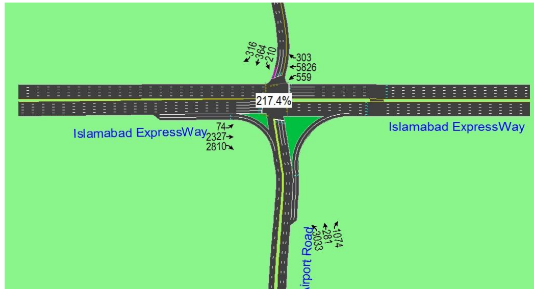
Figure 4.9 Intersection Capacity utilization (ICU) after optimization
