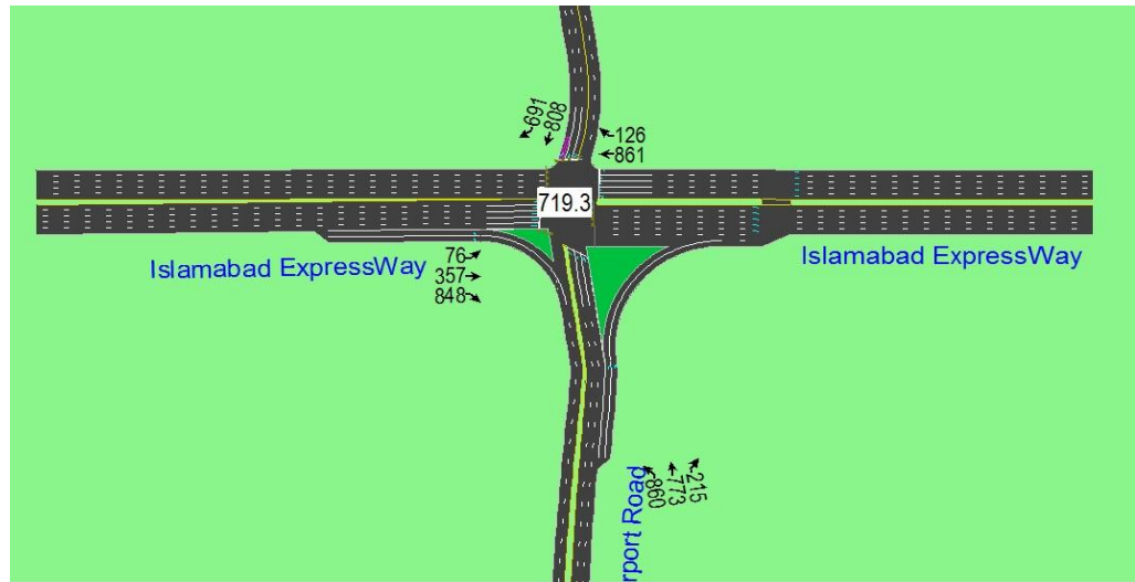
Figure 4.7 Intersection Delays and Movement Delays after optimization
