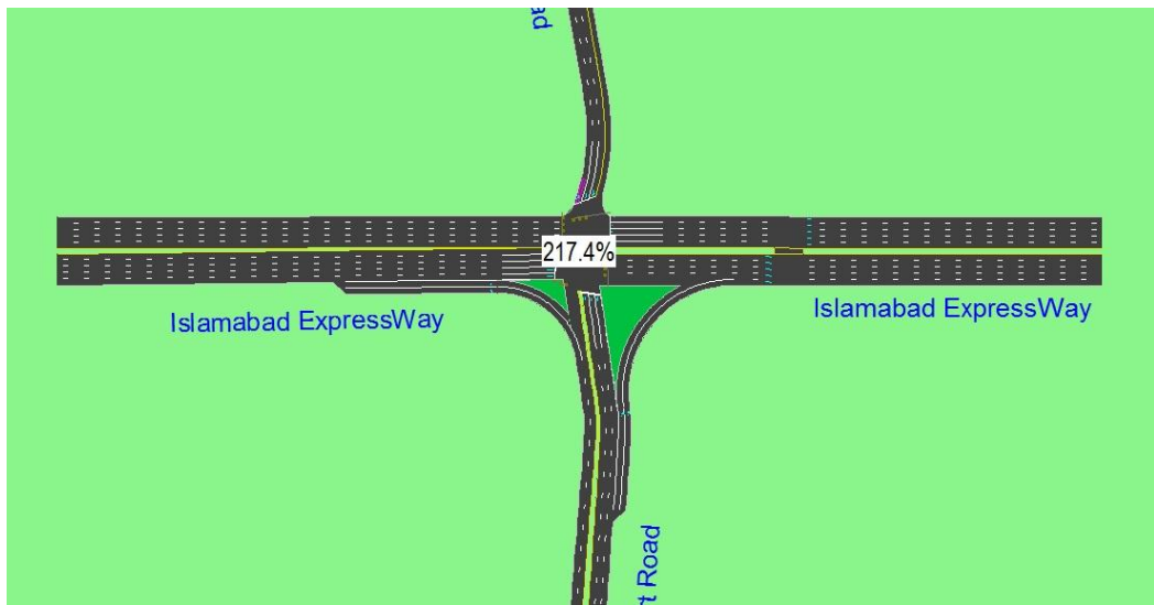
Figure 4.5 Intersection Capacity utilization (ICU) before optimization
