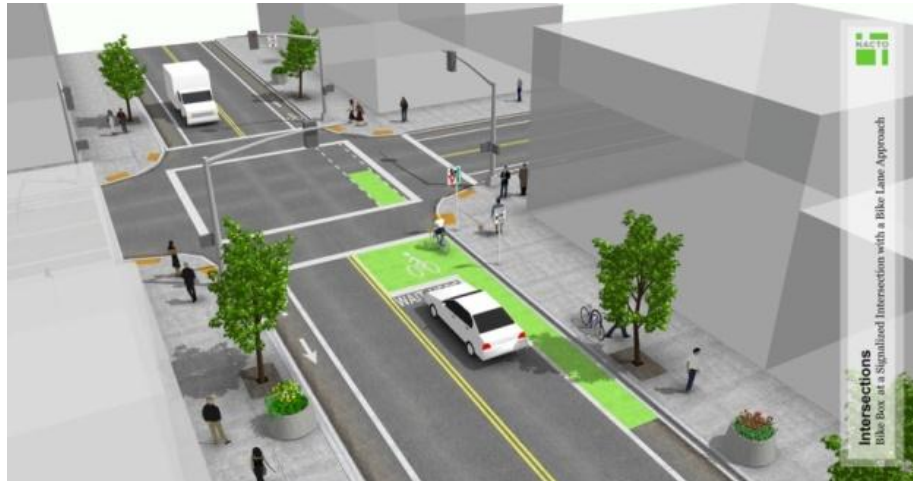
Figure 2.1 At-Grade Urban Signalized Intersection
