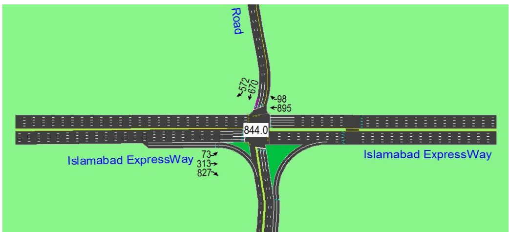
Figure 4.3 Intersection Delays and Movement Delays before optimization
