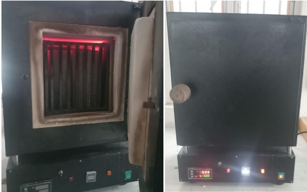
Figure 3: Electric Furnace for heating the samples to targeted temperatures
