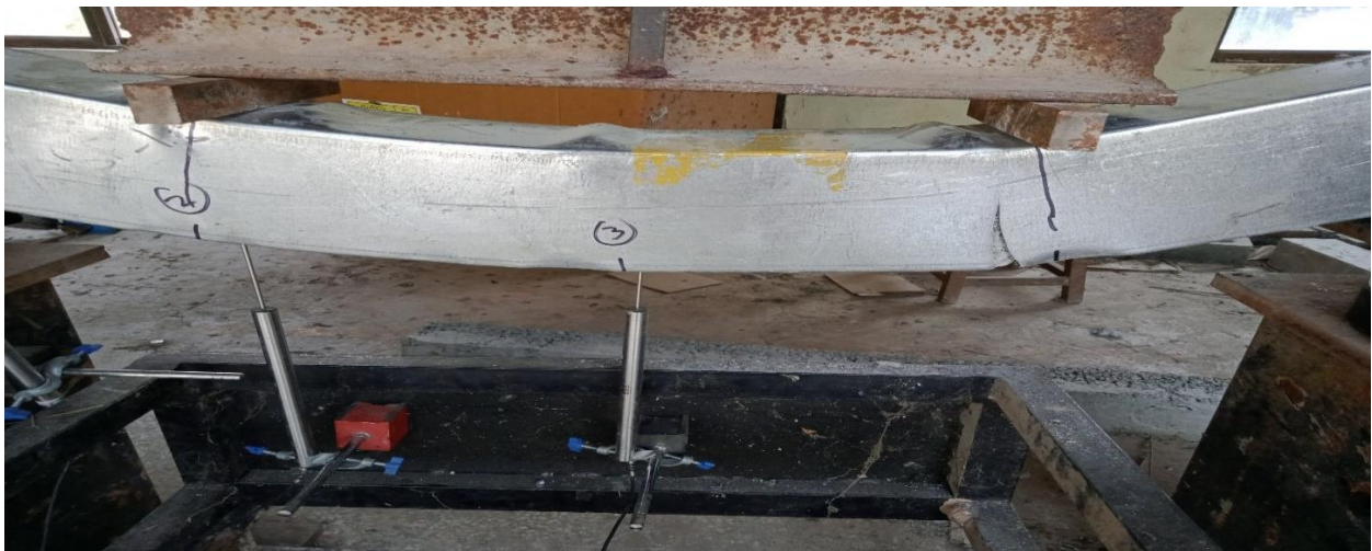
Figure 4.17: Failure pattern of beam with steel fibers reinforcement strengthened with steel sheet (SF-0-S)
