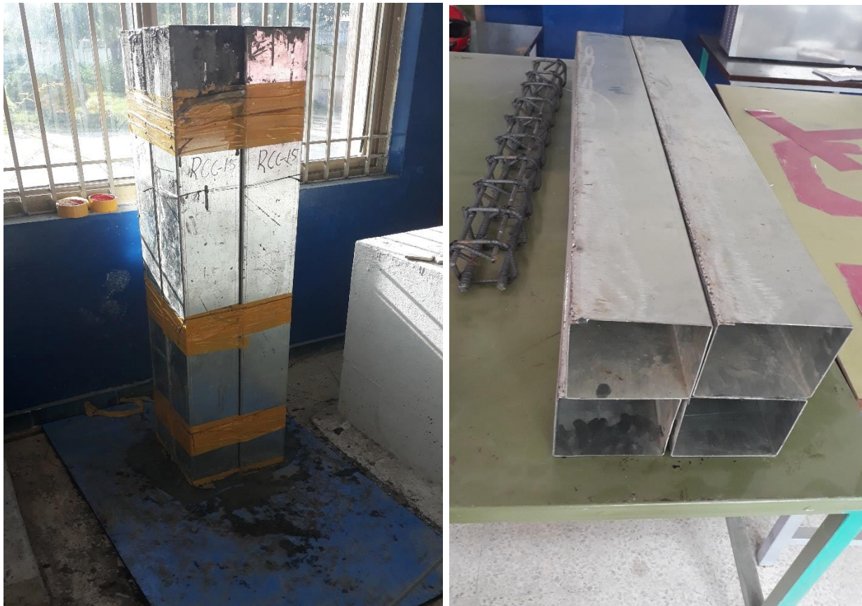
Figure 4.4: Fabrication & Pouring of Steel Tubes
