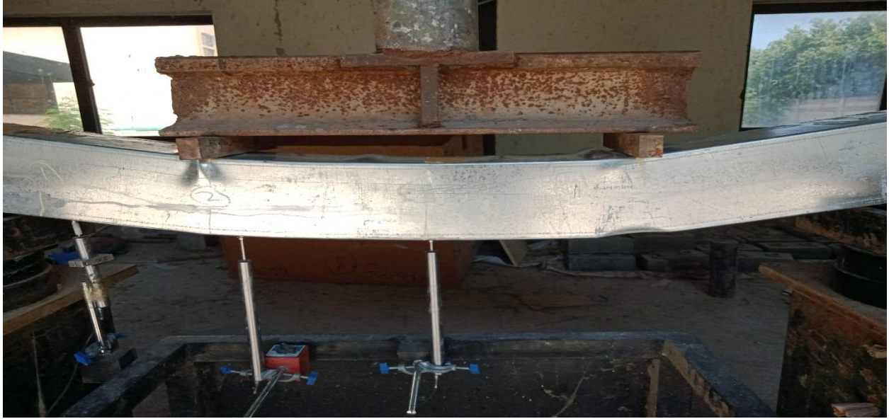
Figure 4.18: Failure pattern of beam with flexural and steel fibers reinforcement along with steel sheet (SF-R-S)
