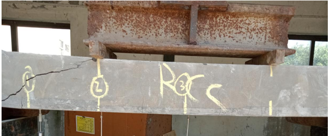
Figure 4.14: Failure pattern of Reference Beam (Ref)
