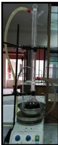
Figure 21: Reflux in oil bath
