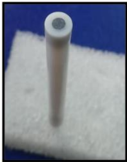
Figure 25: Dried ink on glassy carbon electrode
