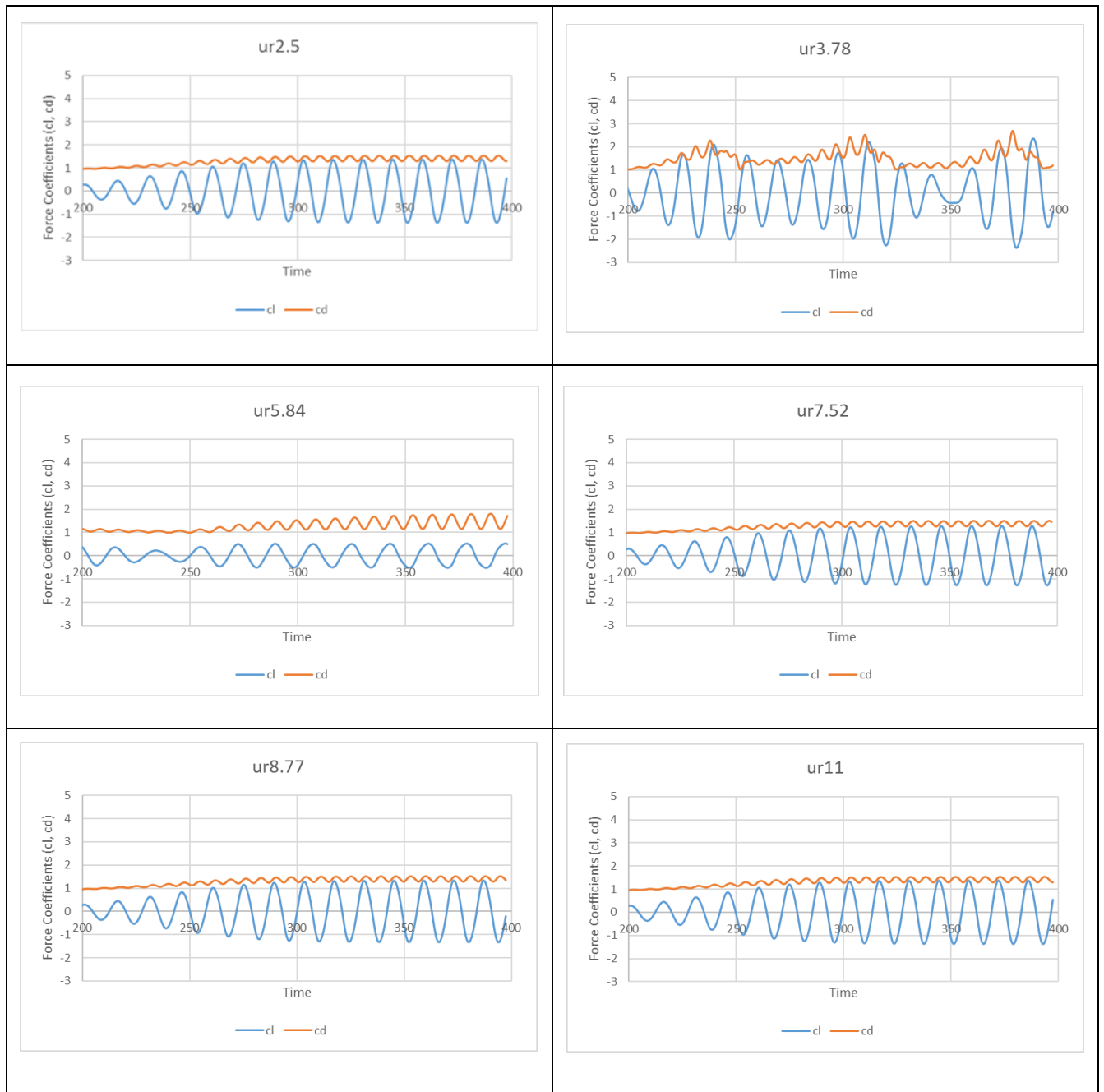
Figure 13. Time history of force coefficients ( c_d & c_l ) at ( U_r=2.5, 3.78, 5.84, 7.52, 8.77 & 11)
