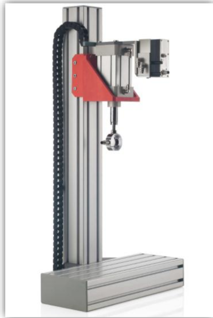
Figure 1: Reference System, LiTem fatigue testing machine
