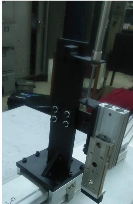
Figure 31 Probe and slider assembly (Manufactured and assembled on the electric slider)
