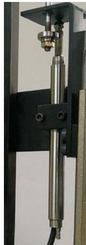
Figure 40 Solartron AT/5/p installed on the machine
