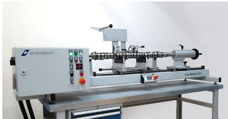
Figure 9 Camshaft driven between two live centers
