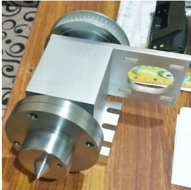
Figure 33 Drive plate (Manufactured and assembled on the drive stock)
